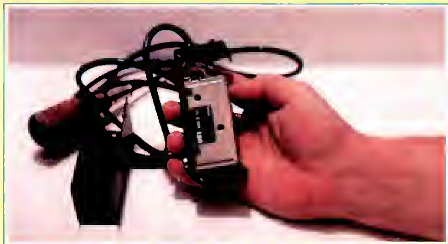
FIGURE 2: Once the box cover has been removed, the modulator itself can be seen and easily accessed for the following steps.
